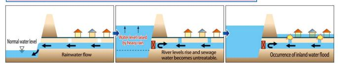
At normal times, the water level of the river to drain water to is low, so rain is drained through sewers (storm sewers). When a river rises due to heavy rain, the river water level rises, and when the water level exceeds the sewer (storm sewer) level, a backflow phenomenon occurs. Therefore, the sluice gate is closed to prevent backflow.
